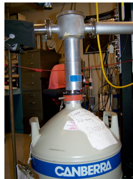
Figure 3: A photo showing the sample analysis chamber, the Ge (Li) detector, and the liquid nitrogen used to cool the detector.
